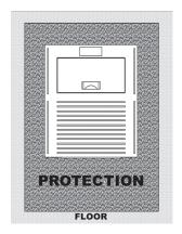
If your flooring is flammable (parquet, floating platform) or sensitive to heat, it is necessary to place a protective layer that separates the heater from the floor.
