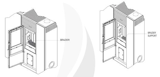
With an ash vacuum cleaner, remove the ashes that have accumulated in the chamber and inside the brazier holder.
