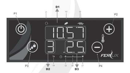
INTERPRETING THE LEDS WHEN THEY LIGHT UP L1 LED lit: the room fan is switched on L2 LED lit: the screw in ON L3 LED lit: the ignition coil is switched on L4 LED lit: ambient temperature reached G L5 LED lit: daily scheduling is activated S LED lit: weekly scheduling is activated L6 L7 W LED lit: weekend scheduling is activated
