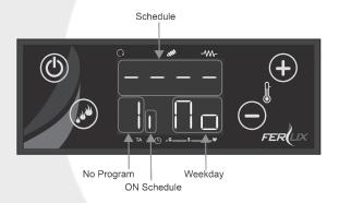
3. After this, long press the (P1) button and on the upper screen (D1), the hours and minutes of the ON state will appear as shown below:
